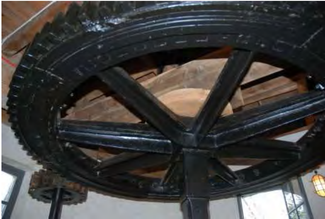
Fig. 70: Photograph of the spur wheel (the large wheel in the foreground) and stone nut (the smaller wheel in the background).
