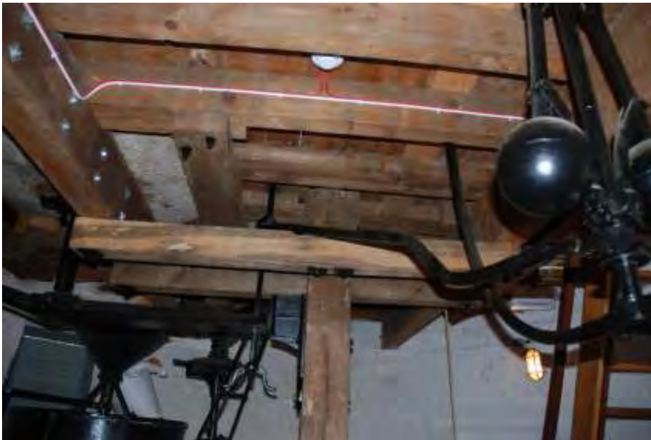
Fig. 84: Photograph showing the governor, and series of levers connecting this to the base of the millstones.
