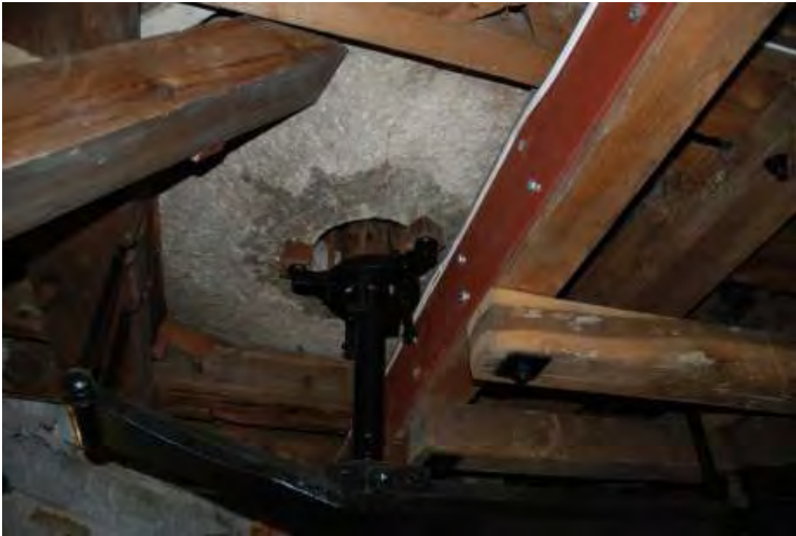
Fig. 85: Photograph of the bottom of the bedstone, viewed from the floor above, and the levers attached to the governor.
