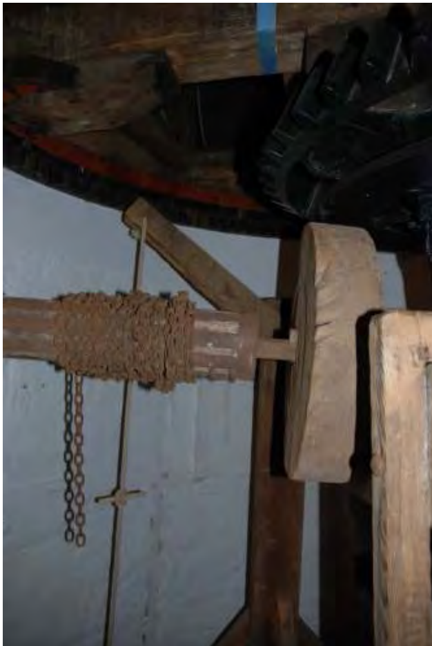
Fig. 64: Photograph of the sack-hoist. The wooden wheel (the 'winch') is visible directly beneath the wallower, with the iron drum leading off this, and the rope and wooden pulley-system behind it.
