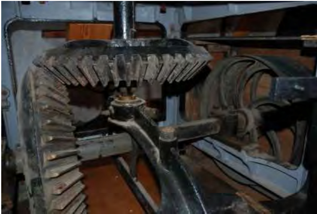
Fig. 89: Photograph of the interior of the provender mill, showing the fan belt (right of image) which is currently driven by electricity, connected to two gear-wheels which rotate the millstones.
