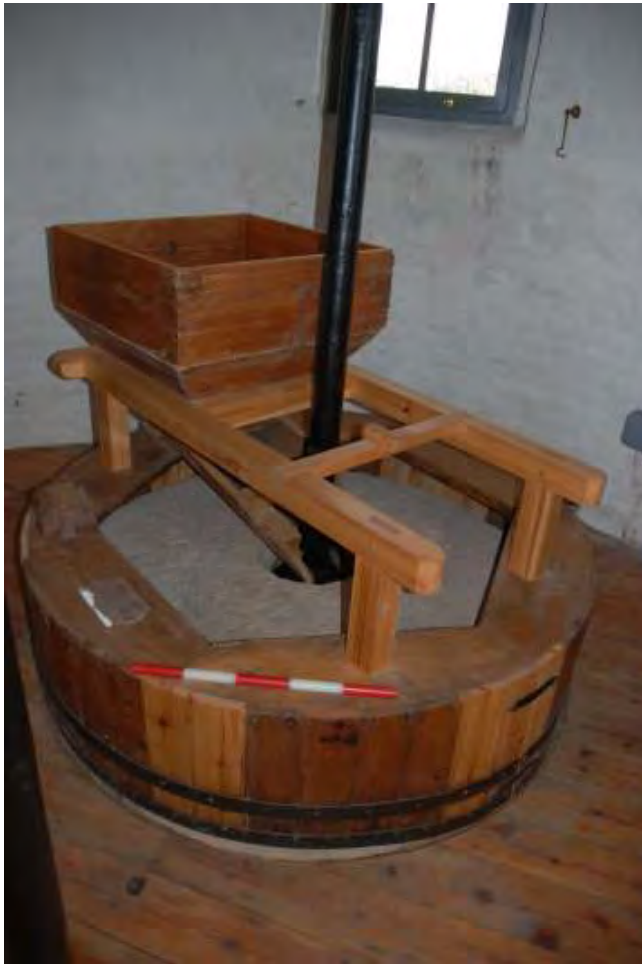
Fig. 72: Photograph of the wooden vat, with the millstones inside, and hopper above.
