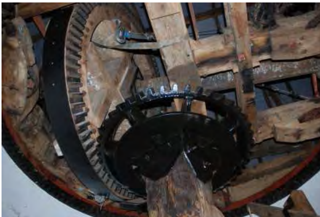
Fig. 62: Photograph looking into the cap. The wallower (the smaller horizontal wheel), brake wheel (larger vertical wheel), and windshaft (horizontal shaft at the top) can all be seen.
