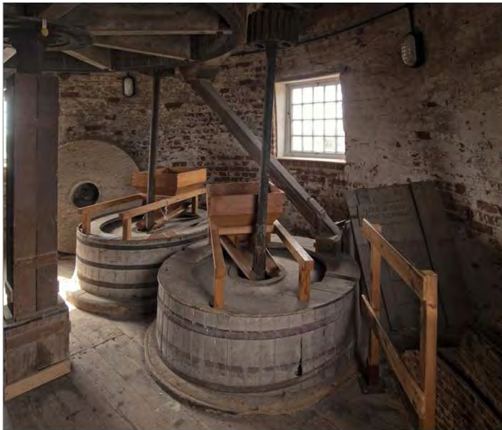
Fig. 96: Photograph of Moulton Windmill in Lincolnshire ( http://4.bp.blogspot.com/-pOOk7O7hptc/T5KoIHPtf4I/AAAAAAAAADmA/XXFPIEjE5TE/s1600/Millstones,-Moulton-Windmill,-Lincolnshire.jpg ), showing two sets of millstones being driven from the same spur wheel. the two stone nuts connected to this single spur wheel can be seen.
