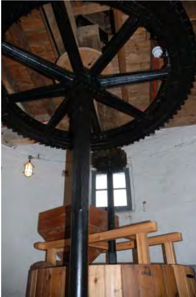
Fig. 71: Photograph of the spur wheel, stone nut, and vat (with millstones in), showing how they are connected.
