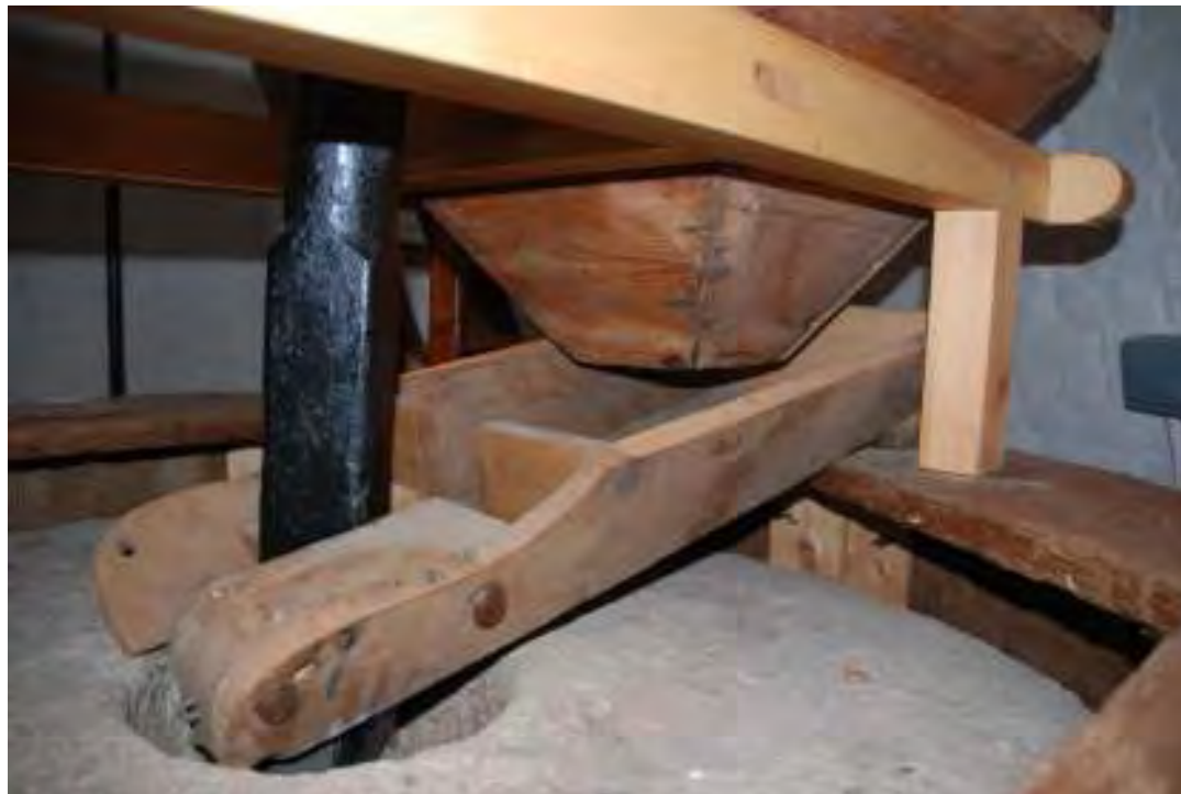
Fig. 73: Photograph of the base of the hopper and the shoe (into which the grain was
