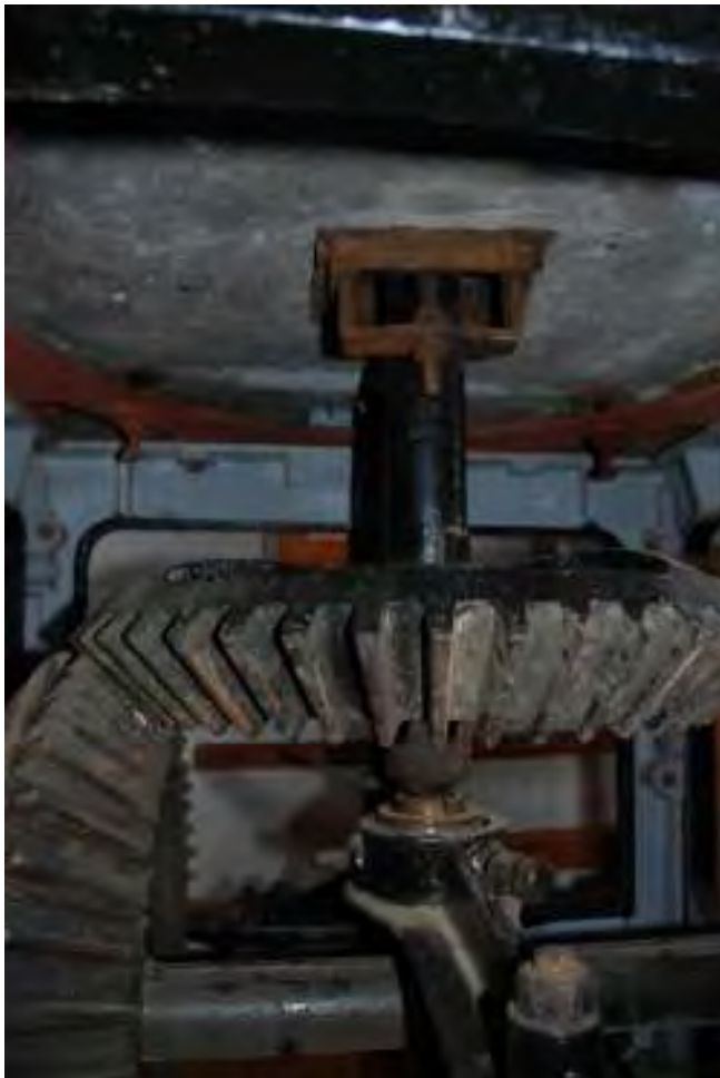
Fig. 89: Photograph of the interior of the provender mill, showing the fan belt (right of image) which is currently driven by electricity, connected to two gear-wheels which rotate the millstones.
